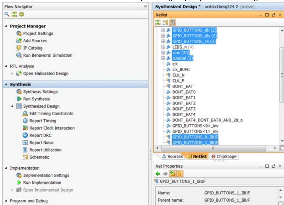
Figure 3: Adding Nets from the Netlist Tab
