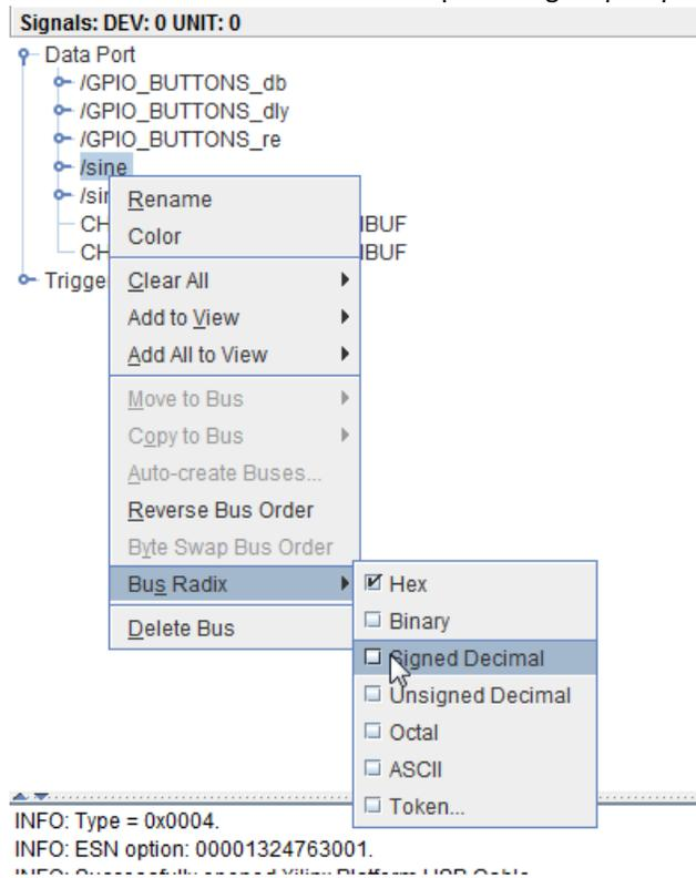
**Figure 10: Changing the radix of the sine signal**
