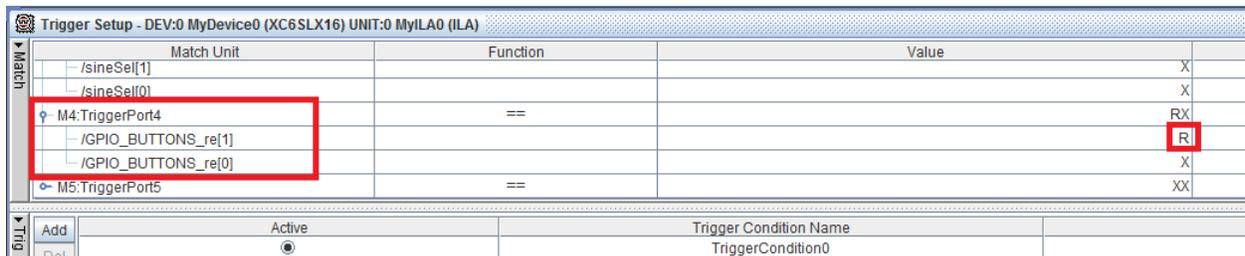
Figure 12: Changing the trigger condition of `GPIO_BUTTONS_re[1]`
